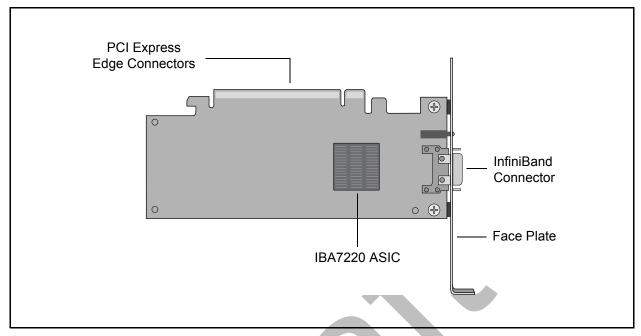
Figure 4-1. QLogic QLE7280 with IBA7220 ASIC
